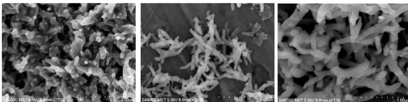
Fig. 6. FE-SEM micrographs of polyaniline nanorods/nanofibers doped with p -TSA
