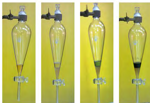
Fig. 2. Photographs of various steps involved during the interfacial polymerization process using separating funnel
