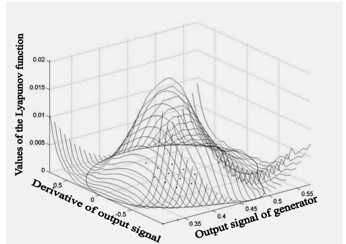
Figure 4. The surface corresponding to Lyapunov function (6). The marked points are the ones, in which additional equations (15) for "soft" excitation of oscillations are composed
