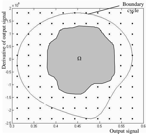
Figure 3. Points – model starting conditions, at which the transient process converges to given boundary cycle. In area  $\Omega$  the oscillations damp
