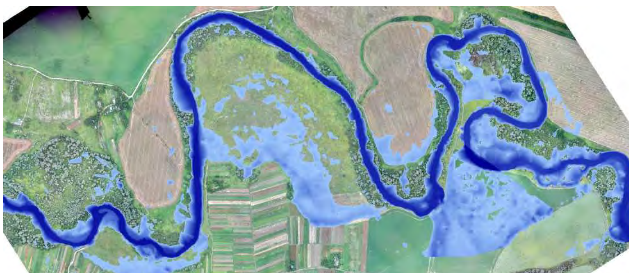
Fig. 10. Flooded area for water discharge 300 \text{ m}^3/\text{s}
