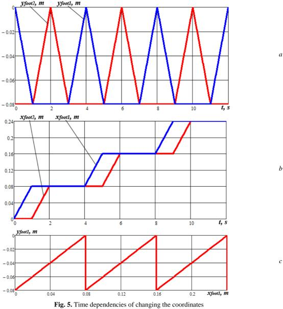
of the robot's supporting feet (a, b) and the motion trajectory (path) of the supporting foot (c)
