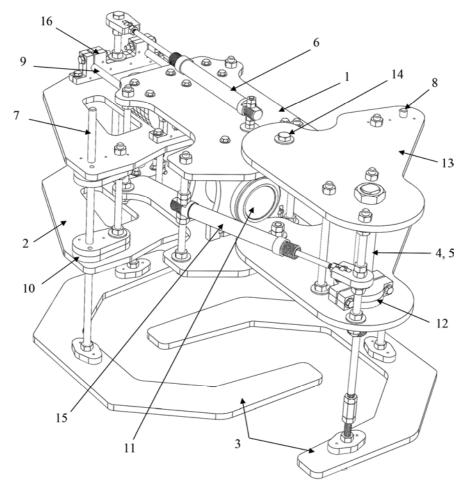
Fig. 1. Improved design of laboratory-scale mobile robot: 1, 2 – movable platforms; 3 – feet;
