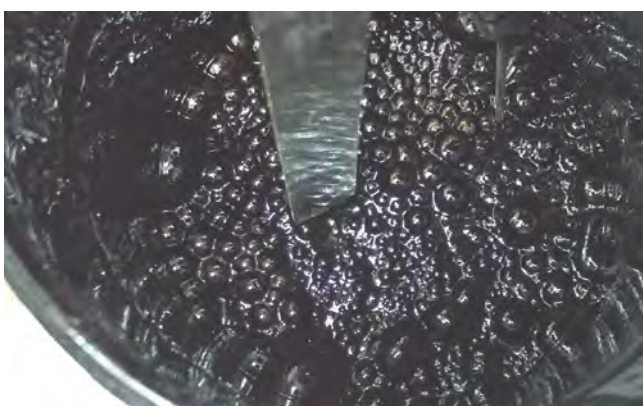
Fig. 2. The process of foaming bitumen by MA
