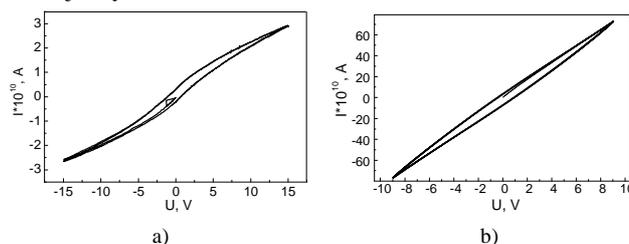
Fig. 1. CVC of detector structures: a)  $\text{Cu-Li}_2\text{B}_4\text{O}_7(\text{X-cut})\text{-Cu}$ ; b)  $\text{Cu-Li}_2\text{B}_4\text{O}_7(\text{glass})\text{-Eu}_2\text{O}_3\text{-Cu}$ . Scanning rate 100 mV/s.
