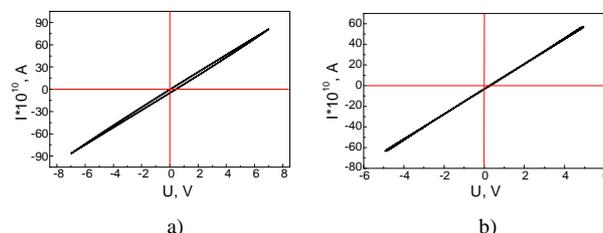
Fig. 2. CVC dependence on the scanning rate: a) 100 mV/s; b) 1000 mV/s. Structure  $\text{Cu-Li}_2\text{B}_4\text{O}_7(\text{glass})\text{-ZnO}(\text{magnetron})\text{-Cu}$ .
