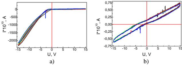
**Fig.3.** CVC of detector structures: a) Cu-Li<sub>2</sub>B<sub>4</sub>O<sub>7</sub>(Z-cut)-Eu<sub>2</sub>O<sub>3</sub>-Cu; b) Cu-Li<sub>2</sub>B<sub>4</sub>O<sub>7</sub>(X-cut)-Eu<sub>2</sub>O<sub>3</sub>-Cu. Scanning rate 100 mV/s.
