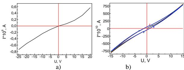
**Fig. 4.** CVC of detector structures: a) Cu-Li<sub>2</sub>B<sub>4</sub>O<sub>7</sub>(X-cut)-ZnO(therm.)-Cu; b) Cu-Li<sub>6</sub>GdB<sub>3</sub>O<sub>9</sub>(001)-Eu<sub>2</sub>O<sub>3</sub>-Cu. Scanning rate 100 mV/s.
