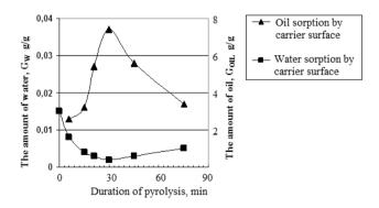
**Fig. 2.** Influence of pyrolysis duration on oil and water sorption of the carbon material ( $T_p = 623$  K)
