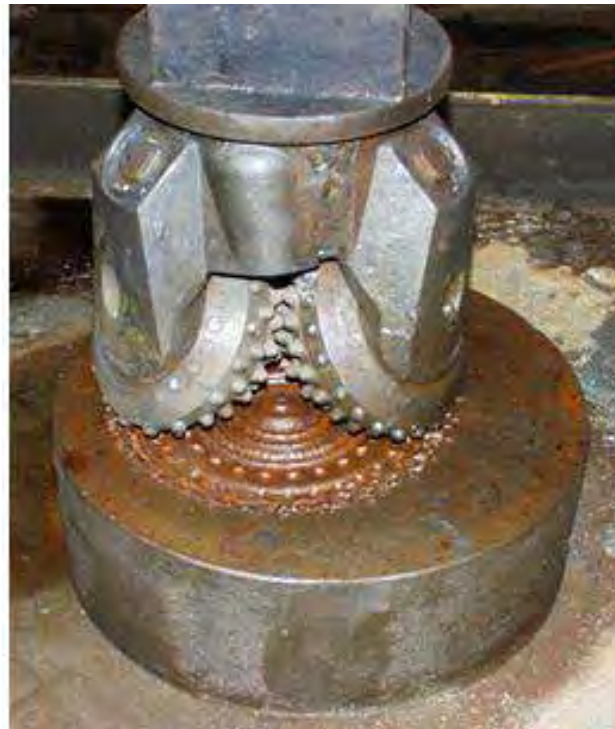
Fig. 2. General view of the tricone drilling bit with experimental rock-destructive inserts after working 8 hours in the stand conditions
