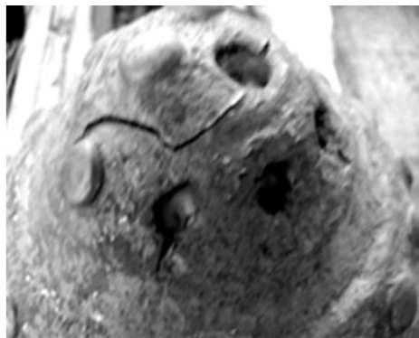
Fig. 1. Macro cracks in the area of the top of the cone and the fall of hard-alloyed cutters
