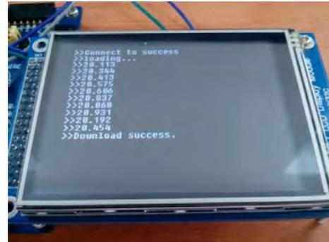
Fig. 5. Display of data array download on LCD.
