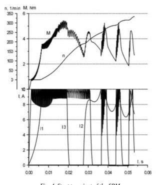
*Fig. 4. Start transient of the SRM with series capacitive energy storage and limited current.*
