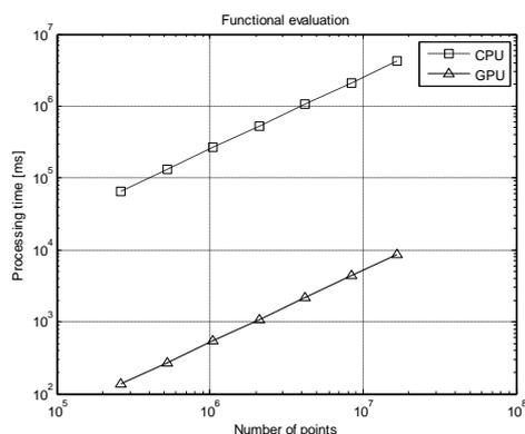
**Fig. 3.** Computation times for the functional evaluation in the sequential and parallel cases.
