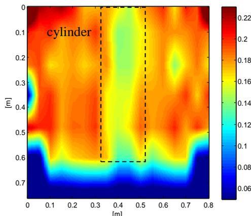
**Fig. 5.** Through-Wall-Imaging of the hidden cylinder.
