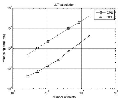
**Fig. 4.** Computation times for the LLT evaluation in the sequential and parallel cases.
