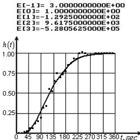
**Fig. 5.** The transitive characteristic and visualization of experimental data on the channel “temperature of the solution at the inlet point of the membrane module – temperature of the solution in a control point on the membrane module length axis”
