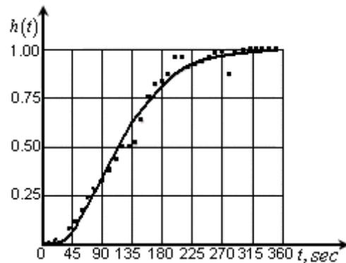
Fig. 4. The transitive characteristic and visualization of experimental data for the channel “heater capacity in the thermostat – temperature of the solution at the inlet point of the membrane module”
