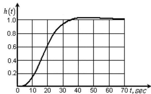
**Fig. 6.** Transitive characteristic of approximated structure
