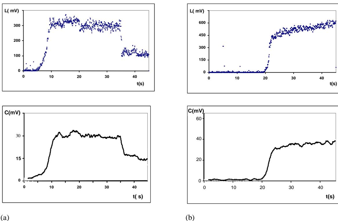
Figure 2: Results of simultaneous recordings the photomultiplier output (SL intensity – upper curves) and the Cavitometer output ( $C$  – lower curves). Ultrasound pulse parameters: pulse period  $T=30\text{ms}$ (a) pulse duration  $\tau=3\text{ms}$
