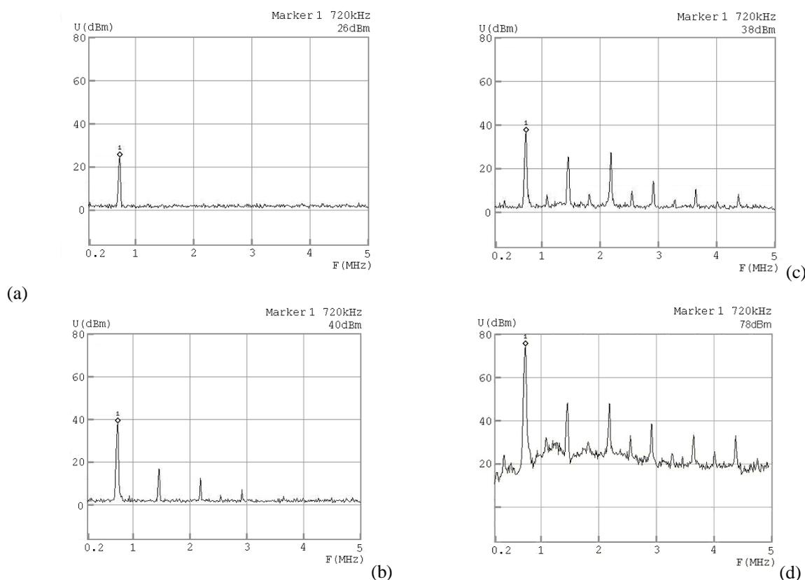
Figure 1: Spectra of the hydrophone output at different stages: stage1(a) below cavitation threshold, stage 2(b) non-linear bubbles pulsation and SL emission appearance threshold, (c)- stage3(c) low intensity SL emission, (d)- stage 4: high intensity SL emission.
