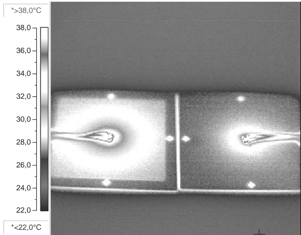
*Fig. 3. Thermovision camera images of heat dissipation of 1mm square resistors on (left) c-BN on alumina and (right) directly on alumina. The resistor was powered with 500 mW*
