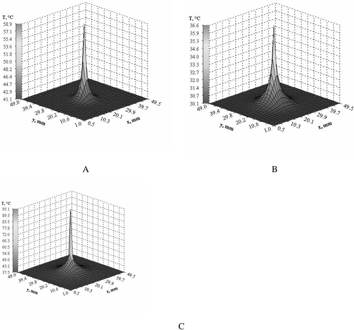
**Fig. 8. Simulation of 3-dimensional heat distribution for a resistor dissipating 0.75W on A – 96 % alumina, B – a layer of cubic boron nitride (c-BN), containing 10% glass on 96% alumina and C – dielectric D421**
