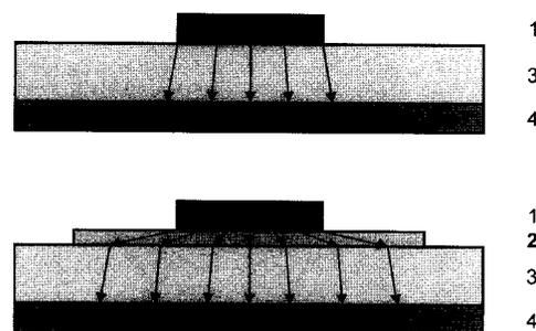
*Fig. 1. The scheme of heat spreading and dissipation through the layers of different thermal conductivity:
