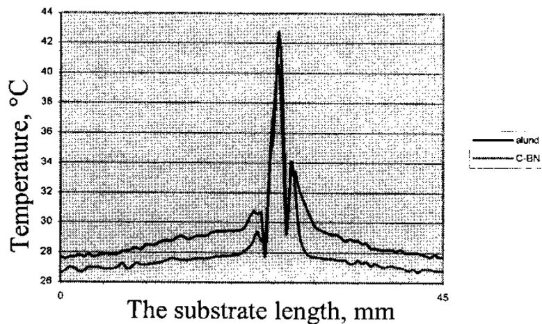
Fig. 5. Temperature distribution along the alumina substrate covered with c-BN layer and on bare alumina with centered resistor powered with 500 mW. The distribution was measured with the use of thermal camera
