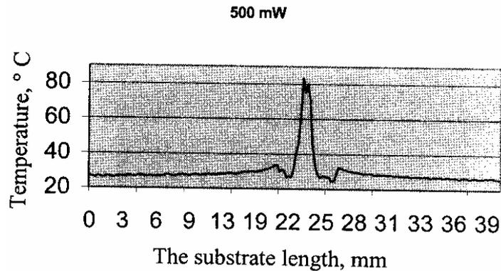
*Fig. 6. Temperature distribution along the alumina substrate covered with dielectric laser D-421 and with centered resistor powered with 500 mW. The distribution was measured with the use of thermal camera*
