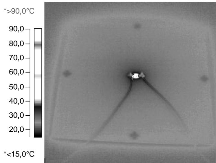
Fig. 4. Thermovision camera images of heat dissipation of 1mm square resistors on D-421 on alumina. The resistor was powered with 500 mW
