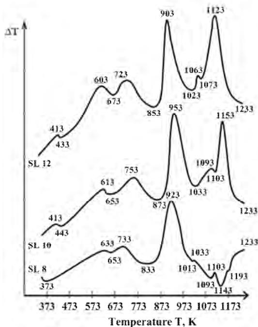
**Fig. 4.** Thermograms of the SL series model glasses
