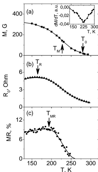
**Fig. 1. Temperature dependences of magnetization in the field  $H = 3$  kOe (a), electric resistance (b) and magnetoresistance in 15 kOe field (c) for the LNMO film. The inset shows  $dM/dT$  as a function of temperature.**
