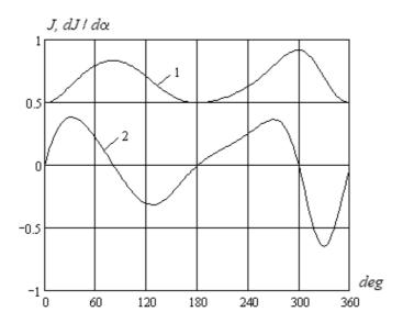
Fig. 1. Inertia moment (1) and its derivative (2) vs. crank rotation angle
