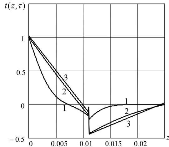
**Fig. 7.** Temperature distributions along the thickness of the composite layer for  $\lambda_1 = 0.5$ ,  $\lambda_2 = 0.8$ ,  $w = -100 \text{ W/m}^2$ . Curves 1–3 correspond to the points of time  $\tau = 10; 90; 360 \text{ s}$ .
