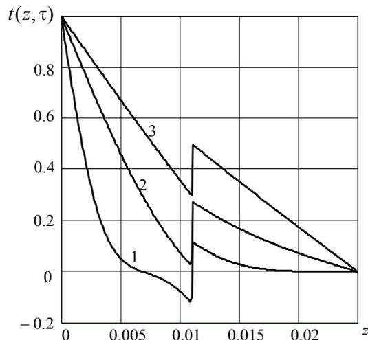
**Fig. 9.** Temperature changes along the thickness of the composite layer. Heat sinks and heat sources are in the vicinity of the interface. Curves 1–3 correspond to the time  $\tau = 10; 90; 360$  s.
