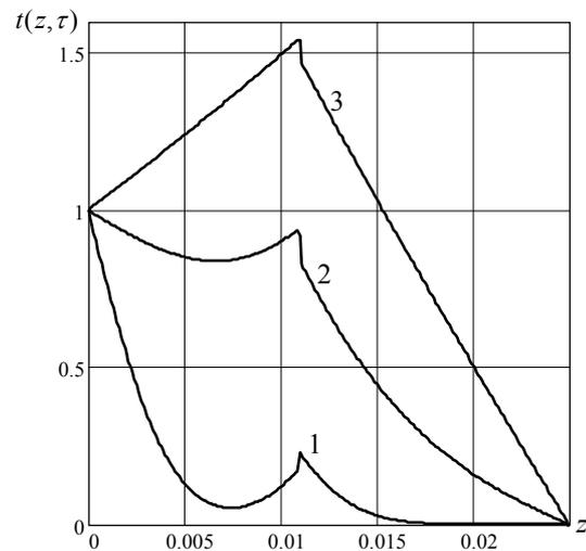
**Fig. 5.** Change of the temperature along the thickness of the composite layer for  $\lambda_1 = 0.8, \lambda_2 = 0.5, w = 100 \text{ W/m}^2$ . Curves 1–3 correspond to the points of time  $\tau = 10; 90; 360 \text{ s}$ .
