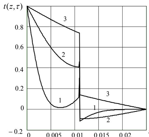
**Fig. 10.** Temperature changes along the thickness of the composite layer. Heat sinks and heat sources are in the vicinity of the interface. Curves 1–3 correspond to the time  $\tau = 10; 90; 360$  s.
