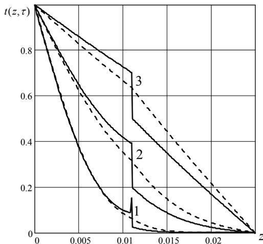
**Fig. 3.** Changes in temperature with respect to the thickness under nonideal conditions of heat transfer (45) between the layers. Curves 1–3 correspond to the points of time  $\tau = 30; 90; 360 \text{ s}$ .
