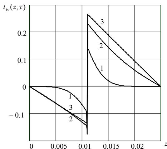
**Fig. 8.** Temperature changes along the thickness of the composite layer. Heat sinks and heat sources are in the vicinity of the interface. Curves 1–3 correspond to the time  $\tau = 10; 90; 360 \text{ s}$ .
