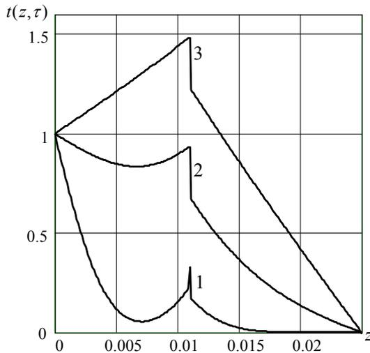
**Fig. 6.** Temperature distributions along the thickness of the composite layer for  $\lambda_1 = 0.5$ ,  $\lambda_2 = 0.8$ ,  $w = 100 \text{ W/m}^2$ . Curves 1–3 correspond to the points of time  $\tau = 10; 90; 360 \text{ s}$ .
