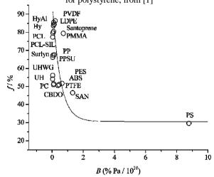
**Fig. 5.** Viscoelastic recovery *f* as a function of brittleness; from [6]. HyAl = Hytrel (a synthetic elastomer) + aluminum; PCL-Sil = polycaprolactone + silica
