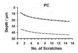
Fig. 2. Penentration depth (the curve with empty circles) and residual depth (the curve with filled circles) for polycarbonate; from [1]
