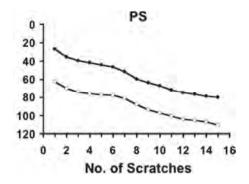
**Fig. 3.** Penentration depth (the curve with empty circles) and residual depth (the curve with filled circles) for polystyrene; from [1]
