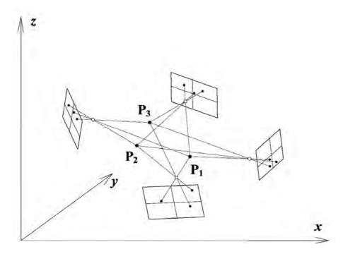
Fig. 6. The principle of convergent photographing
