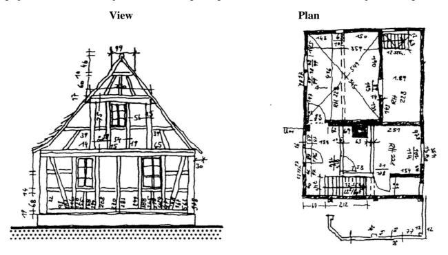
Fig. 1. Handdrawn sketch from the exploration of existing building [1]
