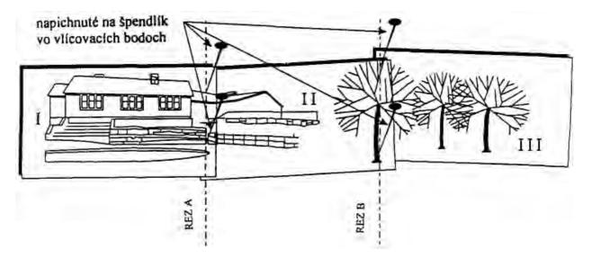
Fig. 3. Scheme of panoramatic photo assamblage out of three pictures (I to III)
