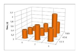
Fig. 4. Reverberation time for frequency f=125[Hz]
