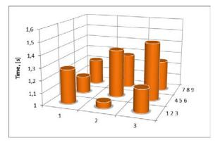
*Fig. 6. Reverberation time for frequency f=500[Hz]*
