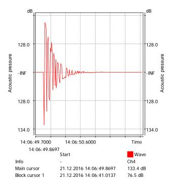
Fig. 3. Acoustic impulse used to estimate reverberation time
