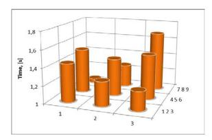
Fig. 5. Reverberation time for frequency f=250[Hz]
