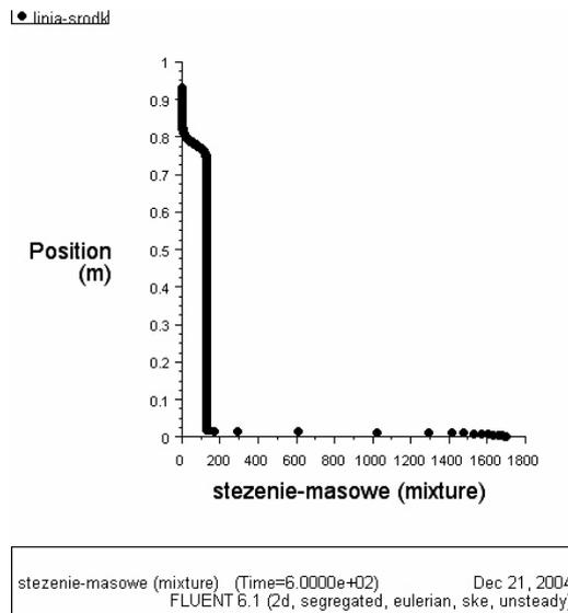
Fig. 8. Schedule of suspension concentration in axis of the cylinder for his vertical setting – Eulerian model – 10 min,
