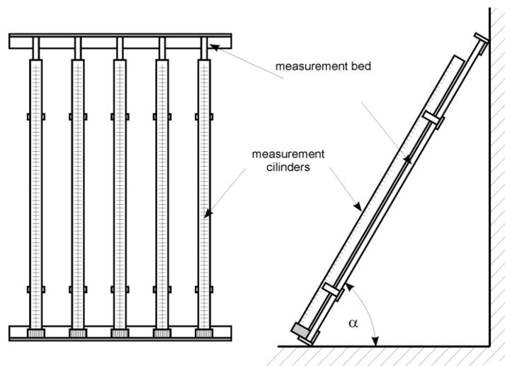
Fig. 2. Stand to the static research of the multiflux concentration process of suspension
