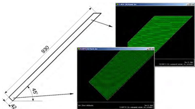
Fig. 4. The system geometry for simulation the static sedimentation and the mesh – inclined cylinder
