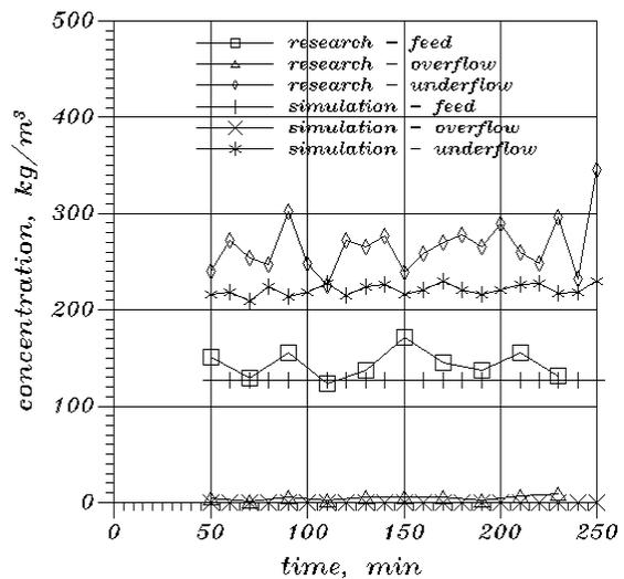
Fig. 19. The feed, overflow and underflow concentration – inclined duct
