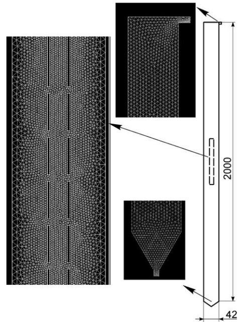
Fig. 17. The geometry to simulation of flow sedimentation in a planar system with mesh
