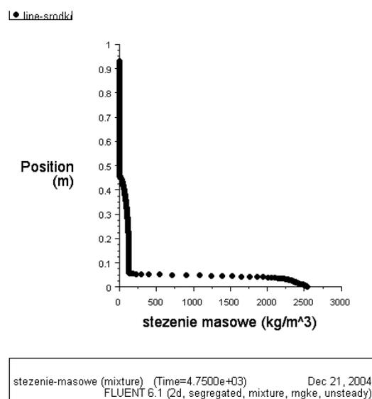
Fig. 7. Schedule of suspension concentration in axis of the cylinder for his vertical setting – mixture model – 80 min
