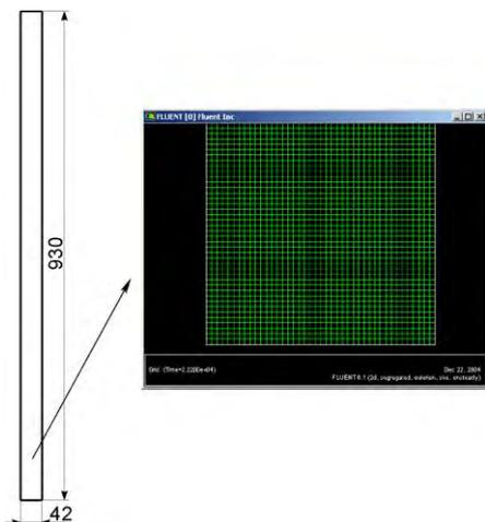
Fig. 3. The system geometry for simulation the static sedimentation and the mesh – vertical cylinder
