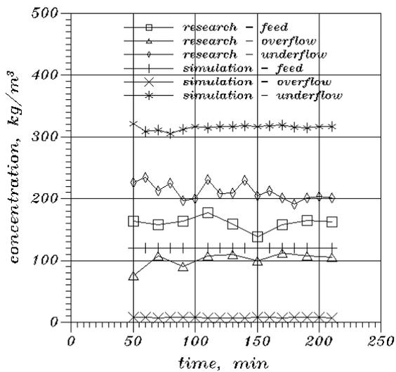
Fig. 18. The feed, overflow and underflow concentration – vertical duct
