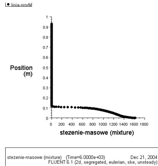
Fig. 9. Schedule of suspension concentration in axis of the cylinder for his vertical setting – Eulerian model – 100 min
