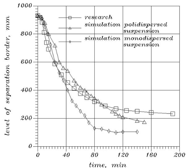
Fig. 15. The sedimentation curve for research and simulations for monodispersed and polydispersed suspension – inclined cylinder
