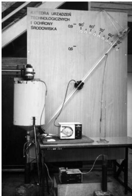
Fig. 16. The laboratory stand to research of flow sedimentation
