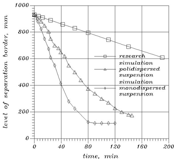
Fig. 14. The sedimentation curve for research and simulations for monodispersed and polydispersed suspension – vertical cylinder
