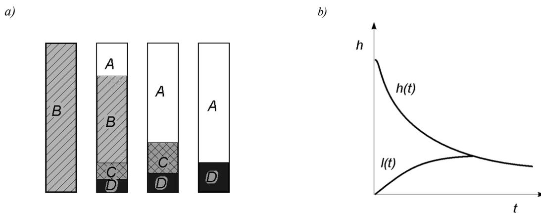
Fig. 1. Course of the periodical sedimentation, a) physical picture, b) the graph of the high of the level separation  $h$  and  $l$  in function of time  $t$
