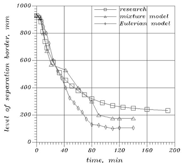
Fig. 11. The sedimentation curve for research and simulations – inclined cylinder
