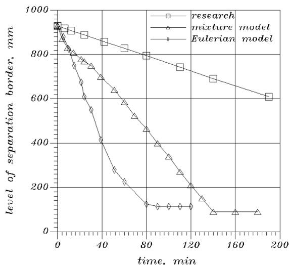
Fig. 10. The sedimentation curve for research and simulations – vertical cylinder
