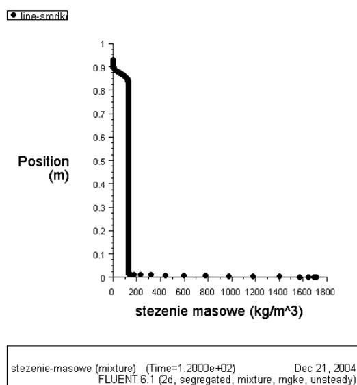
Fig. 6. Schedule of suspension concentration in axis of the cylinder for his vertical setting – mixture model – 2 min
