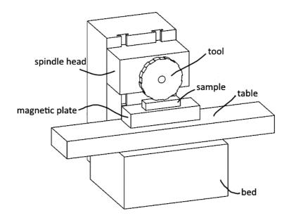
Fig. 1. The model of machine units of flat grinding machine
