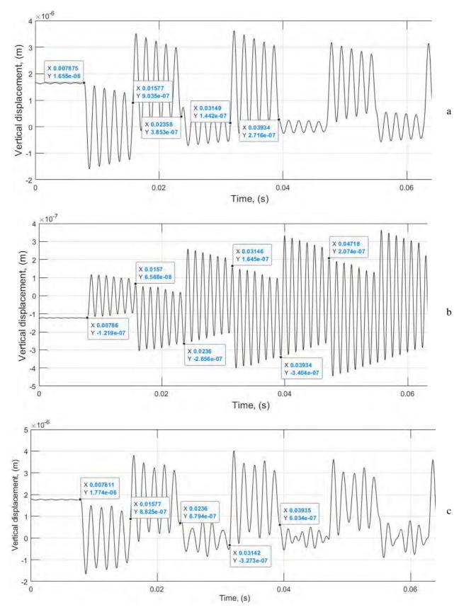
Fig. 9. Displacement the required values: a - displacement the machine spindle in the vertical direction (required value  $x_1$ ); b - displacement the machine table in the vertical direction (required value  $x_3$ );  $c - mutual displacement of the table of machine and part in the vertical direction (required size <math>x_5$ )
