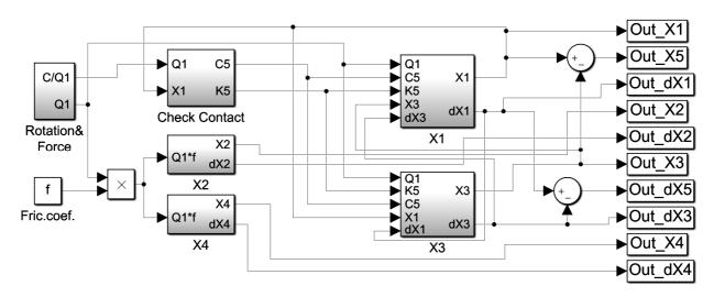
Fig. 4. The block-diagram of simulation model
