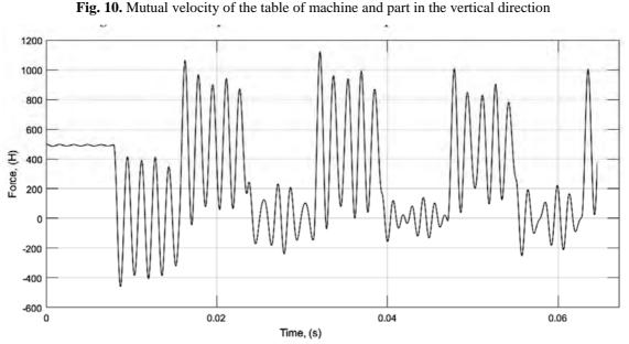
Fig. 11. The interaction force between part and tool
