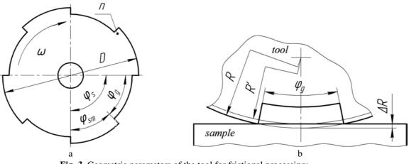
**Fig. 3.** Geometric parameters of the tool for frictional processing: a – sketch of the tool; b – geometry of the groove
