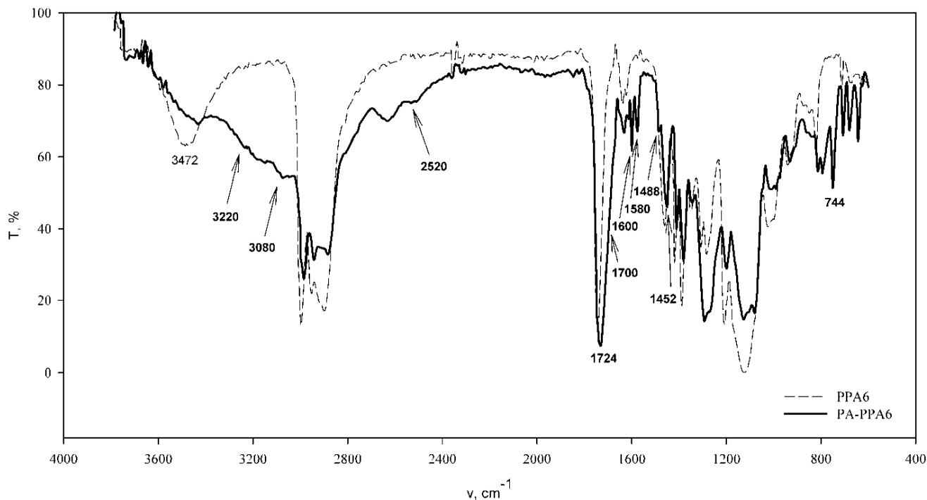
Fig. 13. IR-spectra of PPA6 and PA-PPA6
