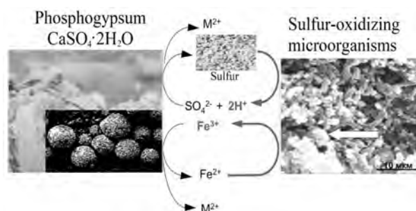
Fig. 6. Granulated PG as a carrier for the growth of sulfur-oxidizing microorganisms
