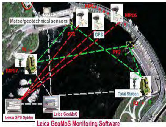
Fig. 3. Scheme of the stationary system for monitoring the spatial displacements of the Dnipro HPP buildings.
