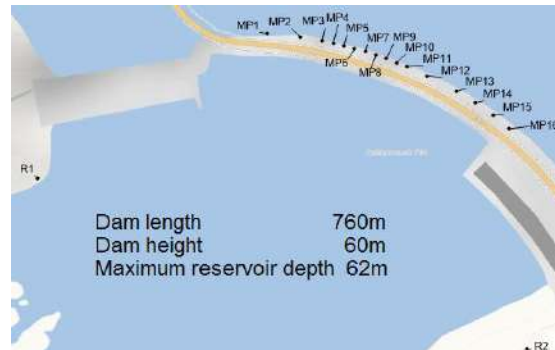
Fig. 4. GNSS network of points on the dam of the Dnipro HPP.
